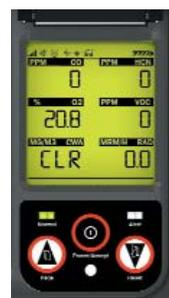
State-of-the-art LCD display provides all six threat readings, LEDs indicate detector status, and keypad allows for alarm acknowledge, sensor calibration, and system setting configuration.
